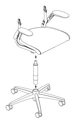
Install the gas cylinder into the 5 star base. Then install the seat assembly onto the gas cylinder.
