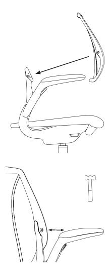
Install the back frame onto the seat frame using the 2 pins. Gently tap the pins using a mallet to securely seat the pins.
