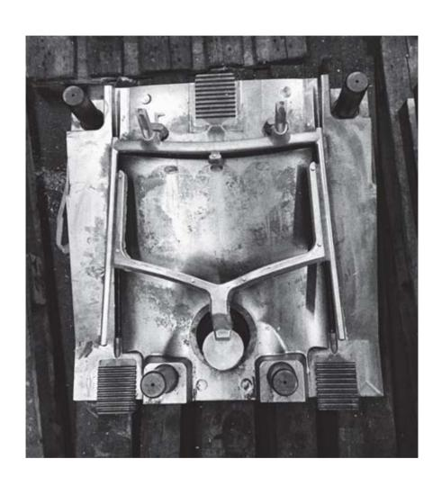
The characteristic lean yet stable shape of the Appia chair is created by the interplay of intrinsic structural elements and advanced mechanical precision. The durable and fully recyclable aluminium frame is produced in a high-pressure die-casting machine and subsequently joined to the oak plywood seat, backrest and optional armrests to create an exquisite surface finish.
