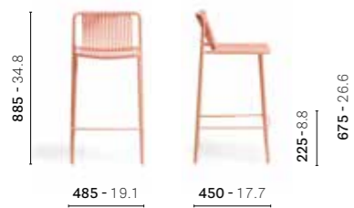
3667 Barstool, steel frame, PVC flexible profile seat and backrest
