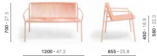
3666 Sofa, steel frame, PVC flexible profile seat and backrest
