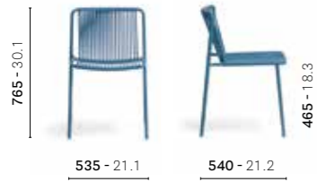
3660 Side chair, steel frame, PVC flexible profile seat and backrest
