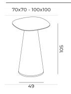
Column weight 19 kg/u Counterweight: Between 12-20kg depends on the table top size Volumetric Packaging 1u. 65,5 x 48,5 x 112 cm
