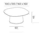
Column weight 13 kg/u Counterweight: Between 25-60kg depends on the table top size Volumetric Packaging 1u. 68 x 57 x 88 cm
