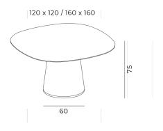
Column weight 37 kg/u Counterweight: Between 25-60kg depends on the table top size Volumetric Packaging lu. 68 x 57 x 88 cm
